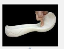
3D printing shoes model for try on (sla soft material)
