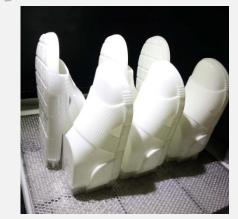
3D printing shoe mold for batch production
