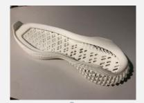
3D printing shoe model for testing appearance and structure (sla hard material)
